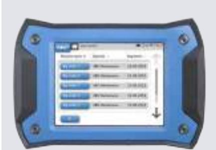
Machine library gives an overview of all machines and alignment reports.
