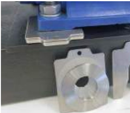
Shims to fix angular soft foot
